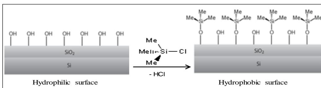
Figure 1: Representation of the modification of chemically oxidized silicon wafers with  $\text{Me}_3\text{SiCl}$ .
