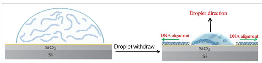
Figure 2: Illustration of the alignment of DNA on the TMS-modified silicon substrate.
