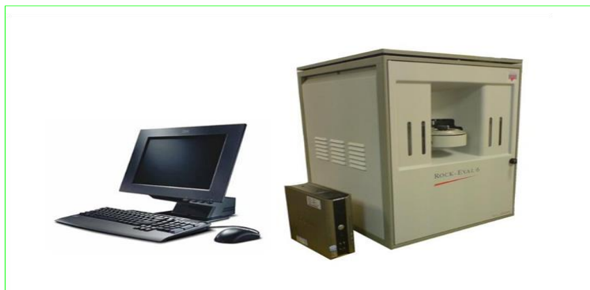
Fig. 2. Illustrative picture showing the Rock-Eval 6 apparatus
